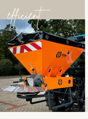
Metal hopper coated with powder paint with enhanced resistance to aggressive environments
